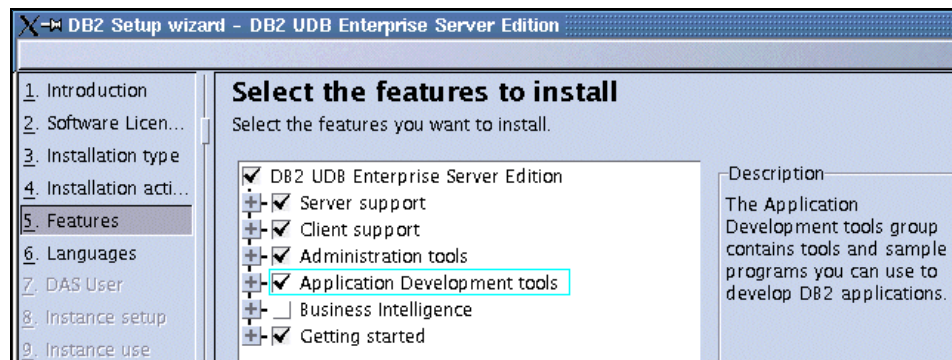
Figure 4-1 DB2 custom installation with Application Development tools selected
